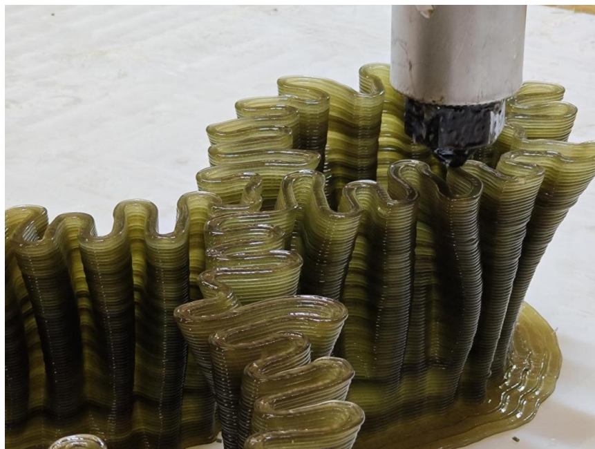
Figure 4. Robotic Fabrication Process of Algal-table 2.0, Photo by Author
